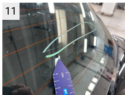
Sted Bagklap Del Bagrude Type Ridser
