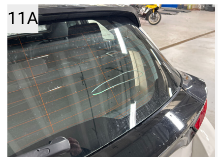
Sted Bagklap Del Bagrude Type Ridser
