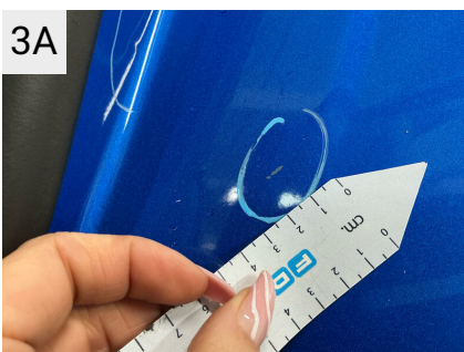
3A Sted V. panel Del Indstigning Venstre Bag Type Bulet/Ridset
