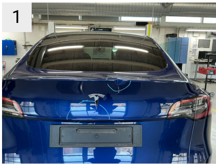
1 Sted Bagklap Del Bagklap Type Bulet/Ridset
