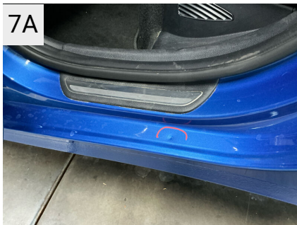
Sted V. panel Del Indstigning Venstre Bag Type Bulet/Ridset
