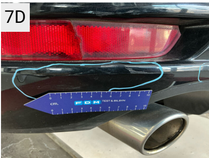
7D Sted Bagkofanger Del Kofanger Type Bulet/Ridset
