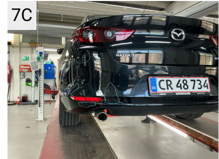
7C Sted Bagkofanger Del Kofanger Type Bulet/Ridset
