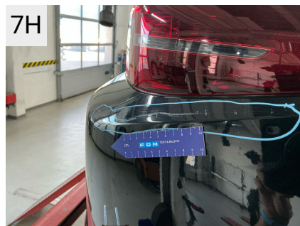
7H Sted Bagkofanger Del Kofanger Type Bulet/Ridset
