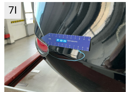
7I Sted Bagkofanger Del Kofanger Type Bulet/Ridset
