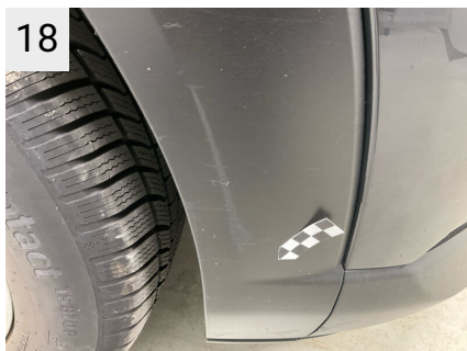
18 Sted Front Del Spoile Type Ridser
