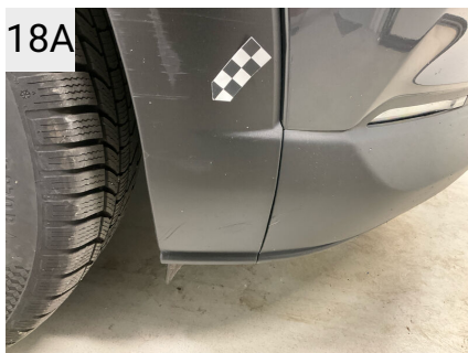
18A Sted Front Del Spoile Type Ridser
