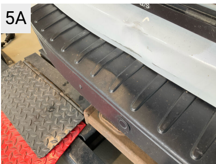
5A Sted Bagkofanger Del Kofanger Type Bulet/Ridset
