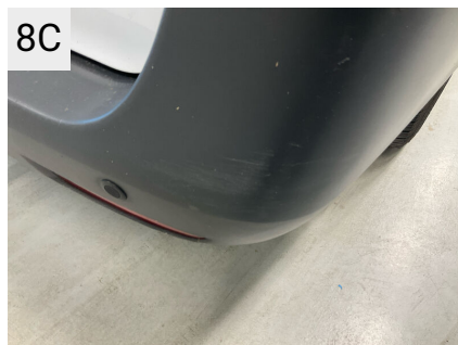
8C Sted Bagkofanger Del Kofanger Type Bulet/Ridset
