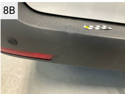
8B Sted Bagkofanger Del Kofanger Type Bulet/Ridset
