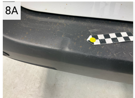
8A Sted Bagkofanger Del Kofanger Type Bulet/Ridset
